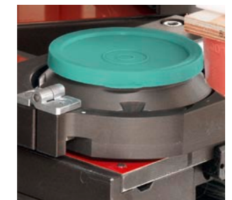
Patented MCI ink cup (compact colour dispensing system)
